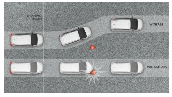
**ANTI-LOCK BRAKE SYSTEM (ABS)** - Be agile in motion as ABS monitors the speed of each wheel to detect and prevent locking.
