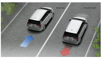
**HILL-START ASSIST CONTROL (HAC)** – HAC temporarily applies the brakes in order to prevent the vehicle from rolling downhill when the driver switches from the brake to accelerator pedal.
